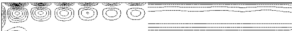
Fig. 14. Isocontour lines of vorticity (left) and isocontour lines of difference between the calculated temperature profile and theoretical conductive one (right), t = 15 , Ra = 40000 .
